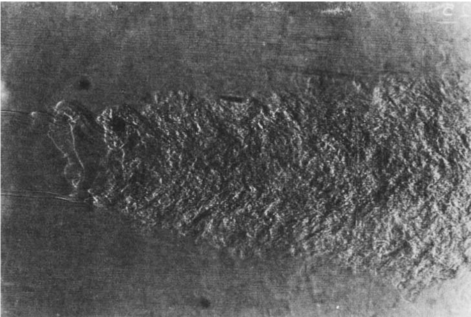
FIGURE 18. Schlieren photograph showing cavitation inception in the core of a vortex.
